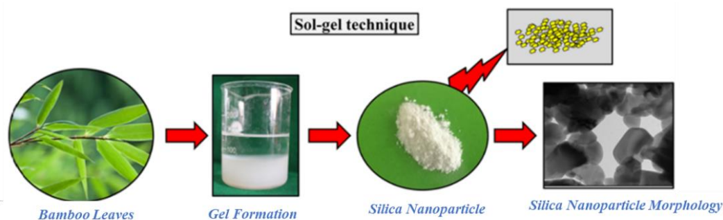
Figure 3. Extraction of Silica Nanoparticles from Bamboo Leaves [26]
