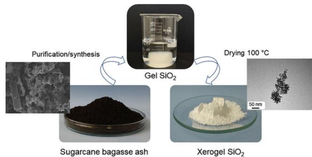
Figure 5. Extraction of Silica Nanoparticles from Sugarcane Bagasse Ash [31]
